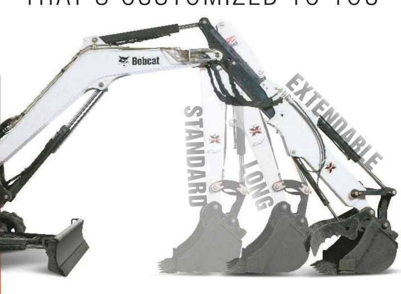
Bobcat compact excavators provide you with the choice of three different lift arm configurations. This allows you to customize the excavator's breakout forces and reach to the work you do most often. Choose a standard arm, long arm or extendable arm.
