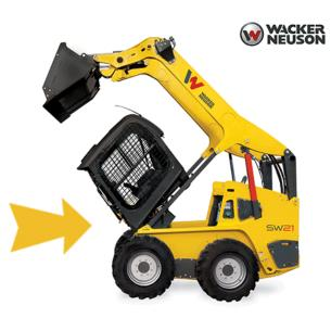
With the cab of the skid steer / track loader flipped forward, a technician is provided with easy and unrestricted access to the hydraulic system.
